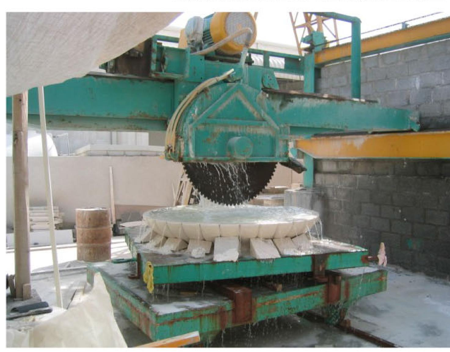
The machine is applicable for producing marble, granite, Stone, Etc. fountain in different sizes and depth.
