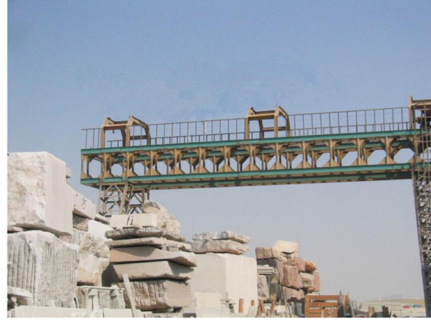
The machine is applicable for handling Blocks, Slab bundle, Container (up to 25 tone safe load).
