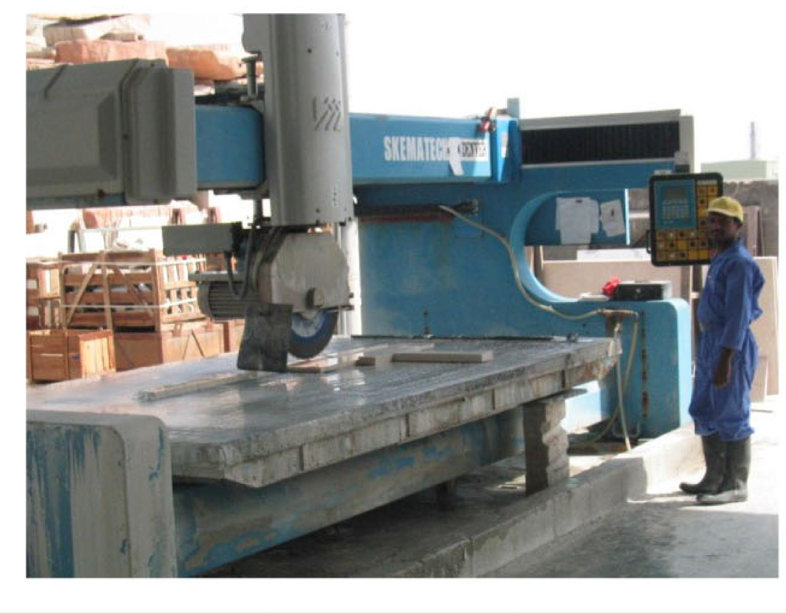
The machine is applicable for cutting marble, granite, Stone, Etc. slabs up to 2 0 c m i n different angles w i t h H i g h efficiency.
