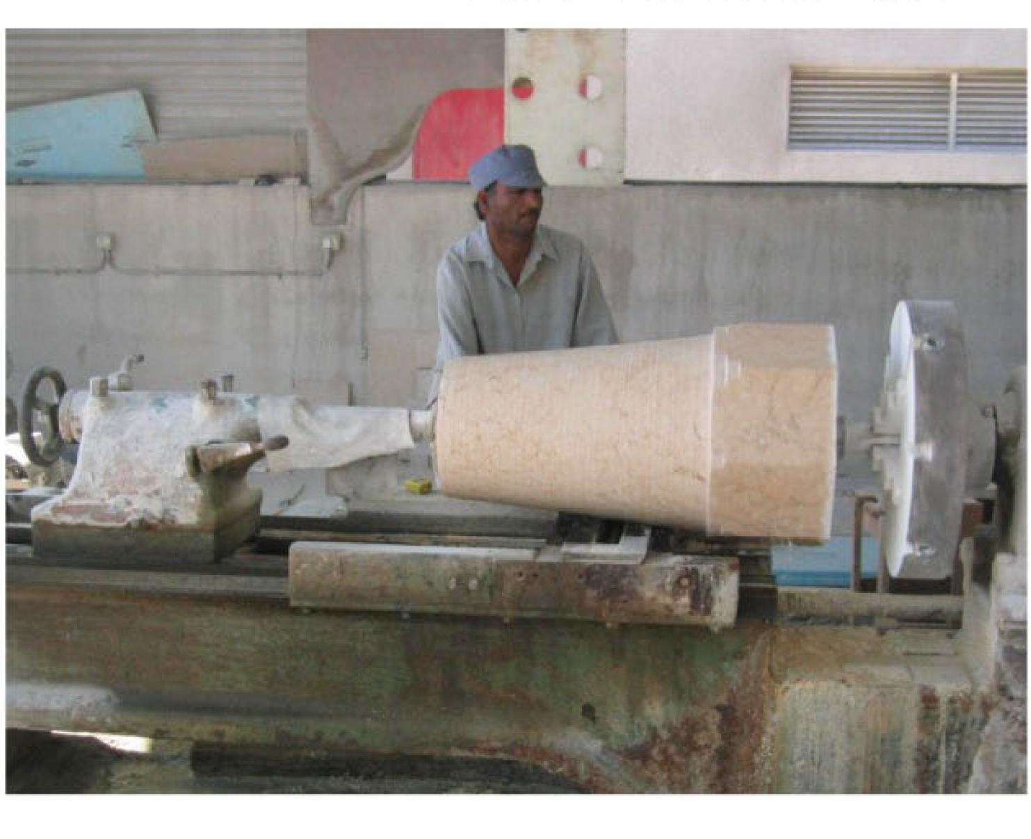
The machine is applicable for producing balustrades, columns, Etc. from marble, granite, Stone.
